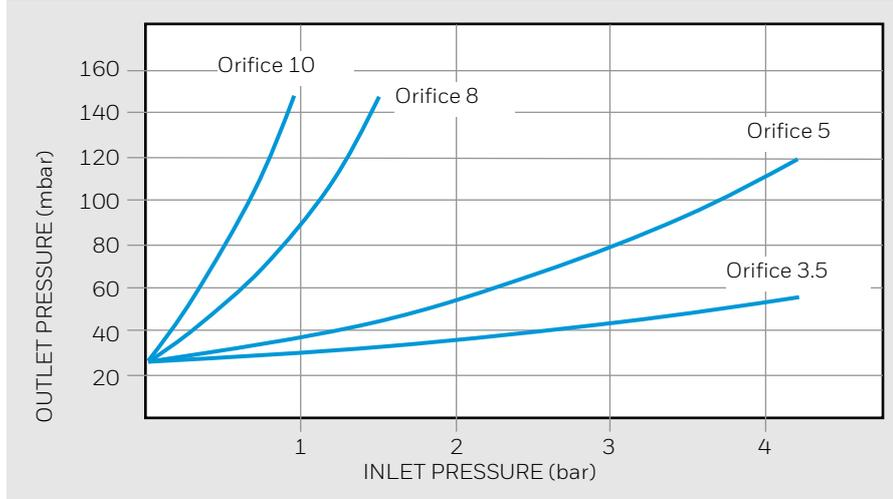
The data represented in the graph left shows the rise in outlet pressure above the set point against change in inlet pressure at a full fault situation.
