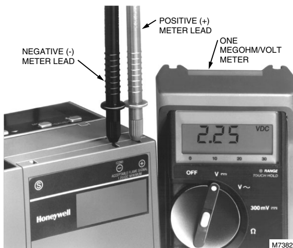
Fig. 18. Flame signal measurement.
