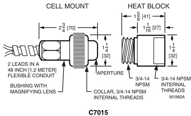
Fig. 6—Ultraviolet detectors (minipeepers).
