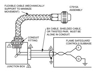
1 BLUE WIRE AND 1 WHITE WIRE FROM THE C7915; CONNECT INSIDE JUNCTION BOX; LEADWIRES FROM JUNCTION BOX NEED TO BE POLARIZED.
