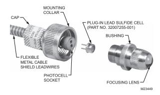
Fig. 8. Installing lead sulfide photocell.
