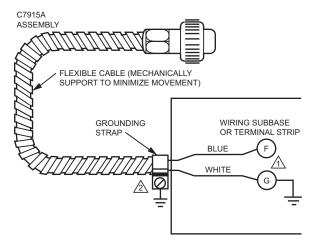
1 BLUE WIRE AND 1 WHITE WIRE FROM THE C7915, CONNECT TO FLAME SAFEGUARD CONTROL'S SUBBASE, KEEP WIRES AS SHORT AS POSSIBLE, AND TWIST THEM.
