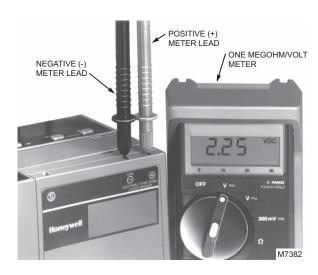
Fig. 12. Measuring 7800 SERIES, R7140 Flame Safeguard Control flame signal voltage.
