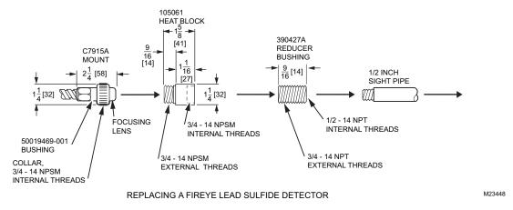
Fig. 1. Mounting dimensions of C7915A Infrared Flame Detector and accessories, in in. (mm).
