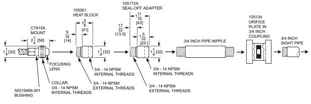
INSTALLING OR REPLACING A C7915A AND ACCESSORIES
