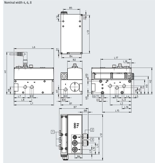
[1] The ports 1, 3, 5 are sealed with the order code D (ducted exhaust air) and F (flat plate silencer).
